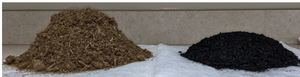
Figure 2. Mass and volume of separated manure solids before and after pyrolysis at 350°C.
