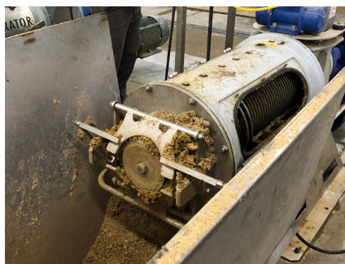
Figure 2. Screw press separator; system positioned to allow solids to collect below the separator (top) and positioned to collect solids in a chute for transfer (bottom).
