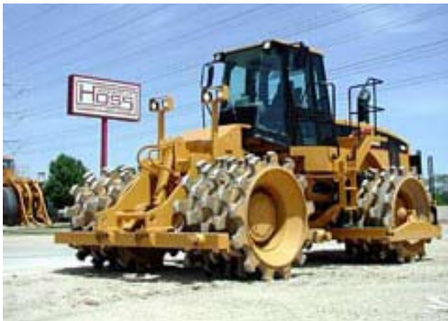
Figure 10D-19 Modern type of tamping roller less well suited for compacting soils for clay liner
