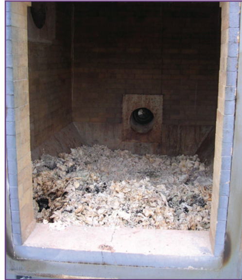
Figure 1. A fixed-facility incinerator (left) and ash from carcass combustion in a fixed-facility incinerator (right). (Courtesy of FC Industries, Inc. Kansas City, MO)
