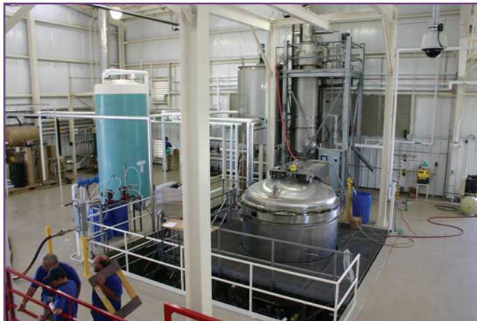
Figure 1. A tissue digester in a fixed alkaline hydrolysis facility. (Photo courtesy of Waste Reduction by Waste Reduction, Inc., Indianapolis, IN)
