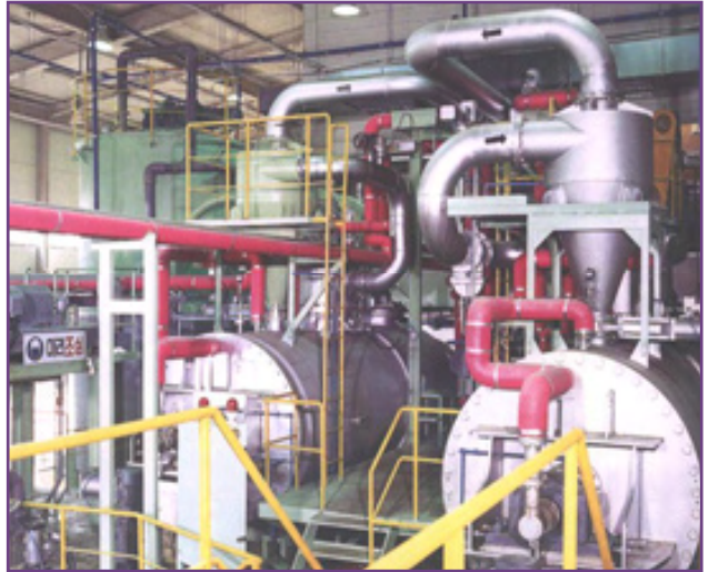
Figure 2. Two views of the equipment used for rendering processes. (Courtesy of Dr. David Meeker of National Renderers Association, Alexandria, VA)
