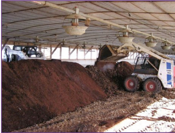
Figure 12. Two views of preparing windrow piles for in-house composting. (Courtesy of Eric S. Bendfeldt, Virginia Cooperative Extension, Blacksburg, VA)
