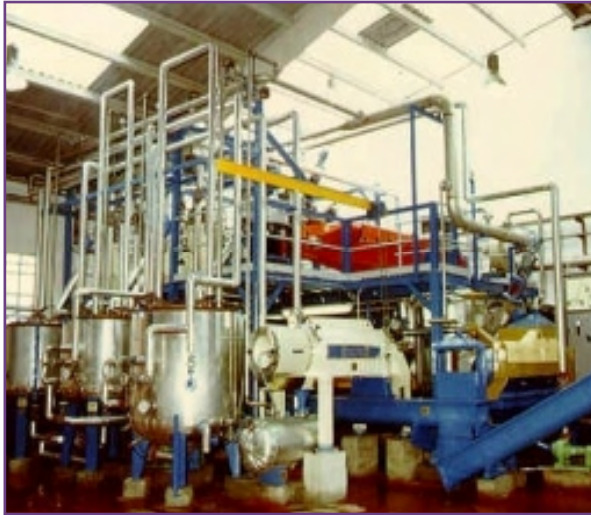
Figure 2. Two views of the equipment used for rendering processes. (Courtesy of Dr. David Meeker of National Renderers Association, Alexandria, VA)
