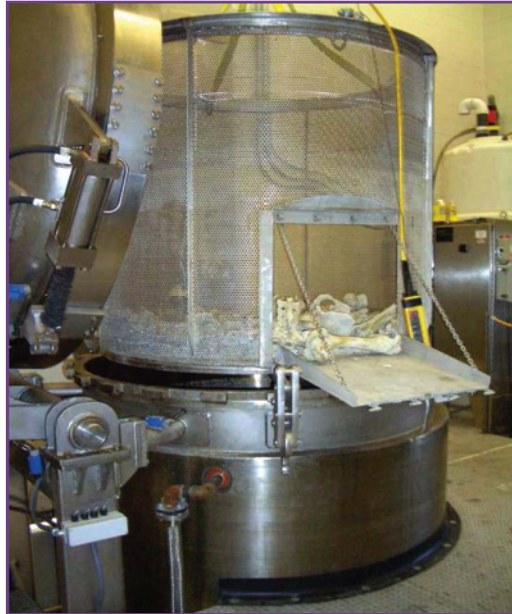
Figure 2. A carcass digester in a fixed alkaline hydrolysis facility. (Photo courtesy of Waste Reduction by Waste Reduction, Inc., Indianapolis, IN)
